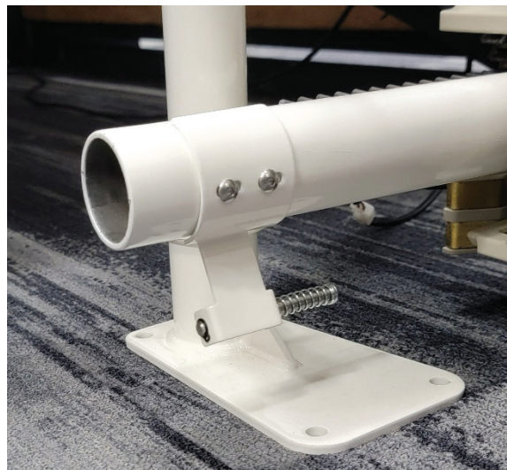
Figure 2.5.5 End Stoppers Installed
