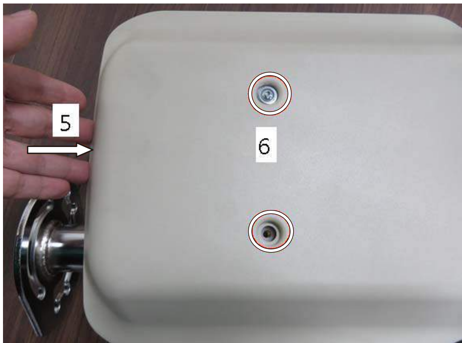
Figure 4-16 Tighten footrest safety cover screws
