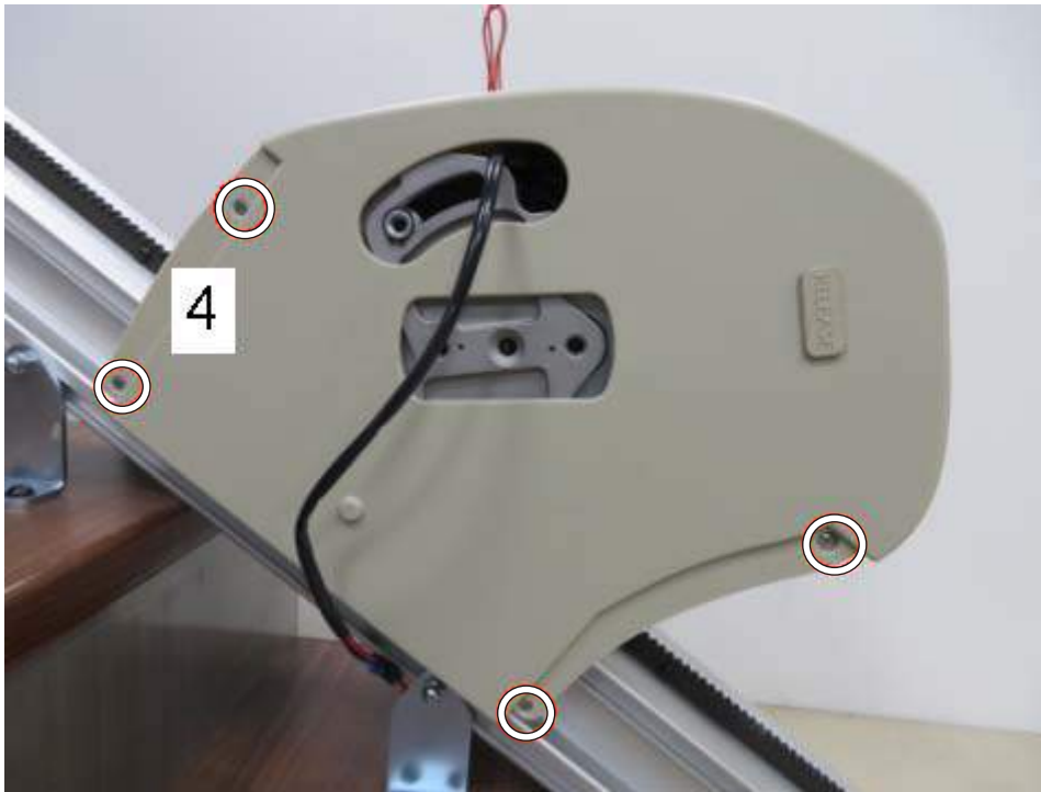
Figure 4-19 Loose screws on the side cover
