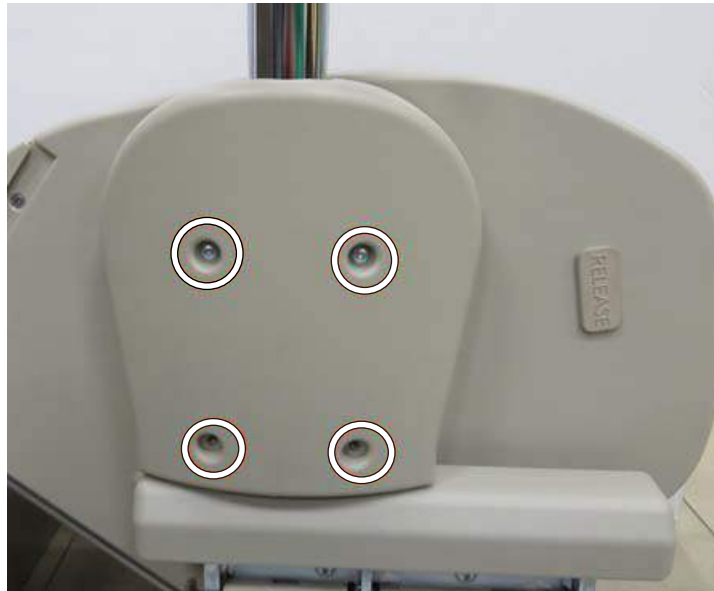
Figure 4-7 Top cover removal
