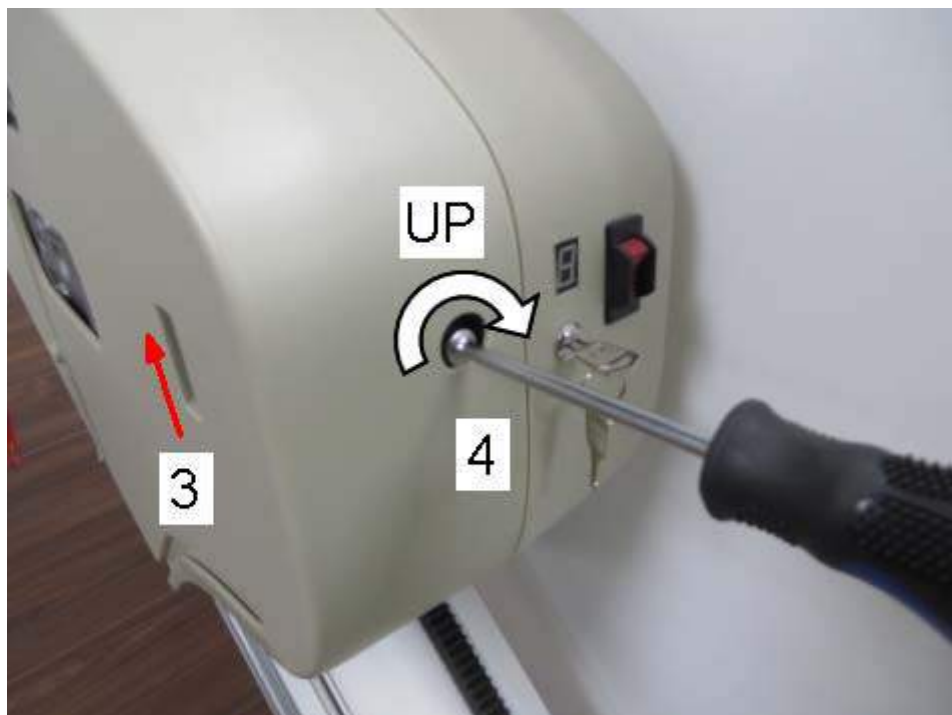
Figure 4-37 Move carriage up by hand crank
