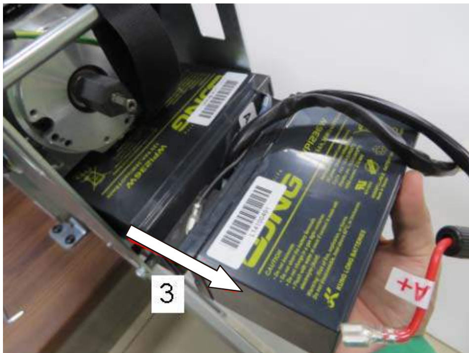
Figure 4-24 Slide the batteries out
