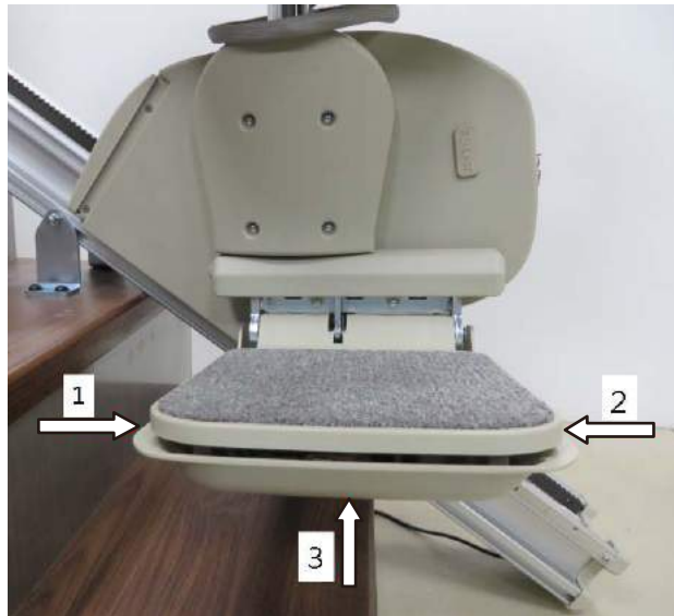
Figure 3-4 Footrest test direction
