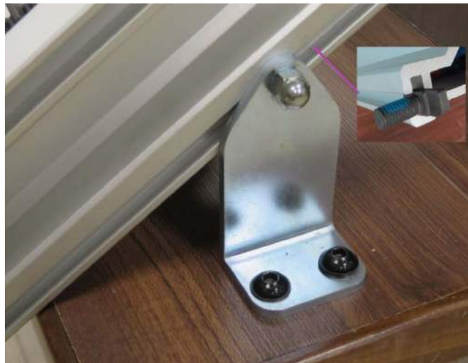
Figure 2-9 Install mounting brackets
