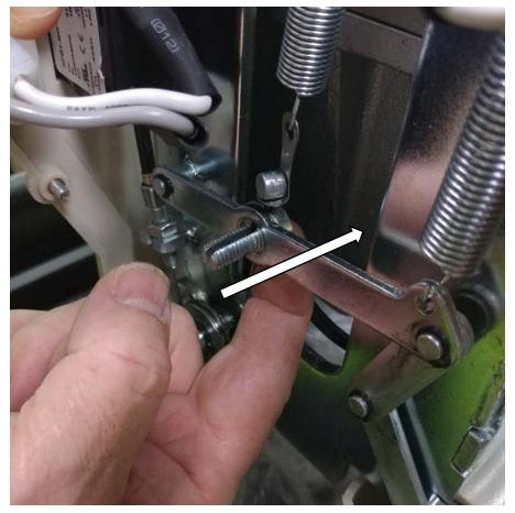
o.) Remove the wire harness of the ON-OFF Switch to enlarge the space for removing the Seat Cable. Separate the Seat Cable and Spring by using a Long-Nose Plier.
