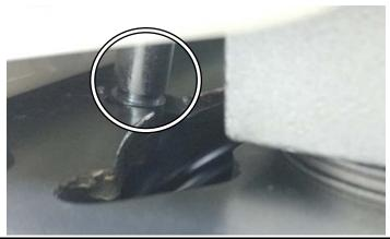
x.) Put the Cable Lead-Head back to the Cable Anchor with the Cable wrapping smoothly around the groove on the Cable Anchor. Knock the Cable Lead-Head slightly back to the recess hole on the Cable Anchor by using a Round Pin.
