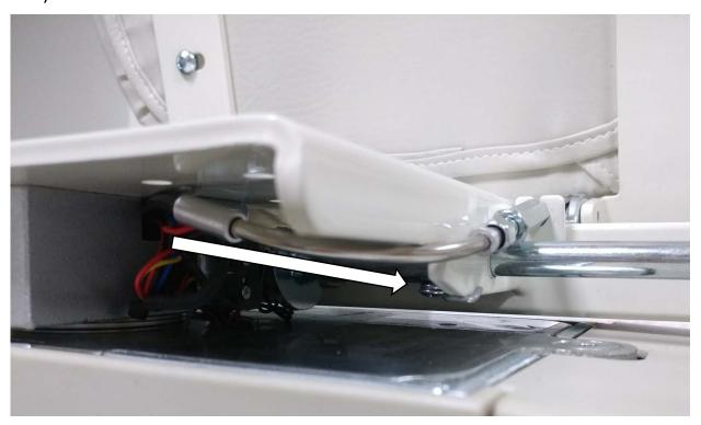
d.) Flip up the Seat half away and pull the Seat Cable in the arrow direction shown below to remove it from the groove on the Cable Anchor.
