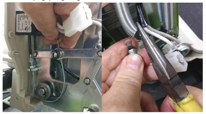
t.) Adjust the Seat Cable to let it wrap around the Cable Pulley. Install the screws beside the Cable Pulley to fix the position of the Seat Cable. Make sure the Seat Cable always remains in the groove on the Cable Pulley.
