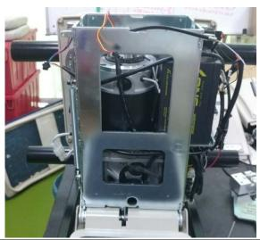
m.) Remove the Nuts on the Footrest Lever by using 2 no. 12 Open-End Wrenches.
