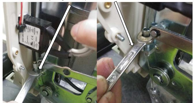
Follow the following procedures carefully to install a new Seat Cable. r.) Let about half of the Cable Screw remain on the outside of the Thread Plate while installing a new Seat Cable.
