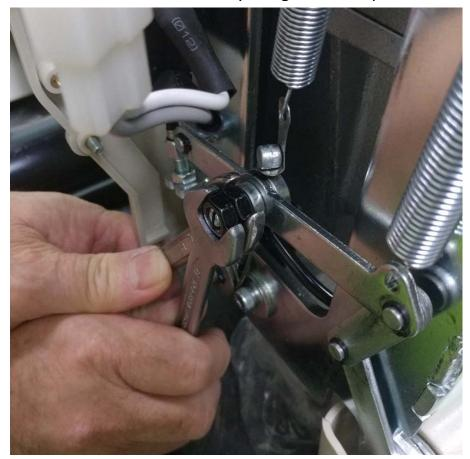
n.) Remove the Seat Cable Screw from the Lever in the arrow direction shown below.
