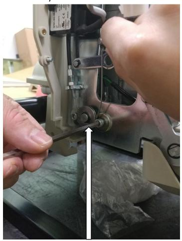
u.) Install the Front Cover, LH/RH Obstacle Sensor Covers, and then LH/RH Covers back to the Carriage. Insert the 2 wire harness and Seat Cable back through the hole of Seat Post. Insert the 2 wire harness first before you insert the Seat Cable.
