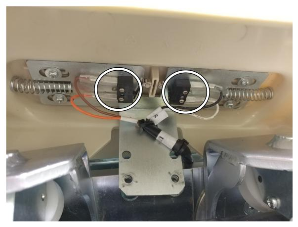
e.) Remove the screws that fixed with the Swing Arm Cover. Replace the old cover with a new one. Install back the screws, Springs and then insert the connectors back to the Limit Switches. Adjust the wire harness and tighten it with Cable Ties.
