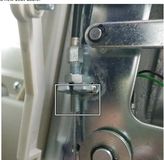
s.) Insert the Seat Cable back to the Seat Cable Screw and lock it with nut. Connect the Seat Cable to the Spring by using a Long-Nose Plier.
