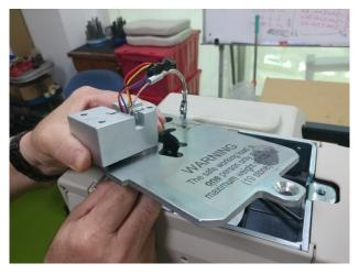
k.) Remove the LH/RH Carriage Covers. Make sure to remove all the wire harness connected on them before removal.
