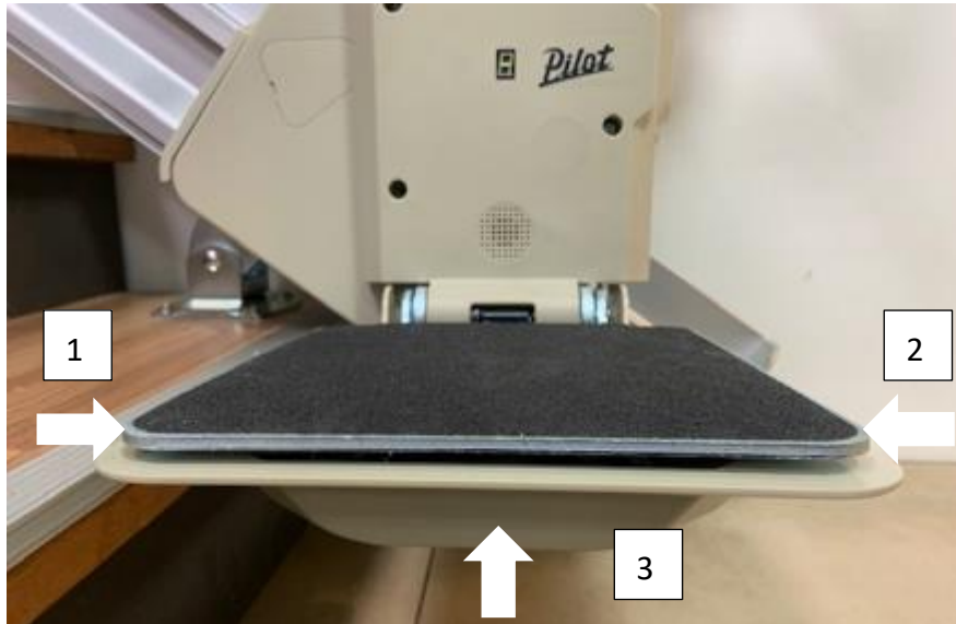
Figure3-2 Footrest test direction
