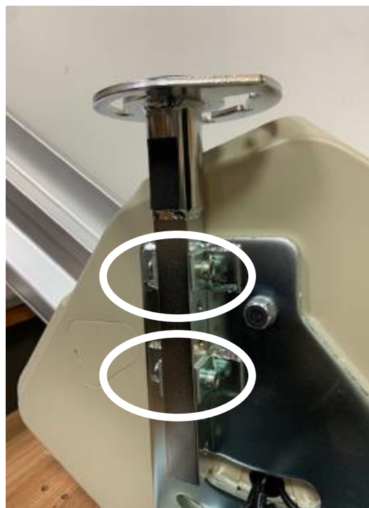
Figure2-17 Seat height adjust
