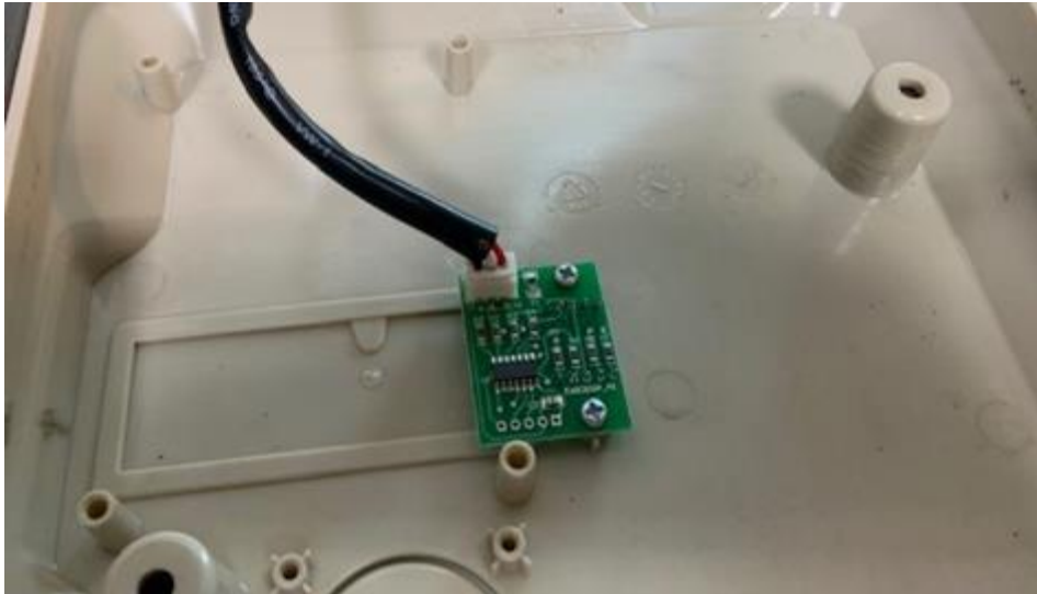
Figure 2-20 cable connect to the board
