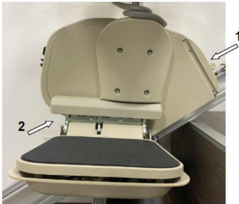
Figure 3-4.1 Carriage Obstacle Sensor Testing
