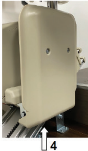
Figure 3-3.2 Footrest test direction when folded
